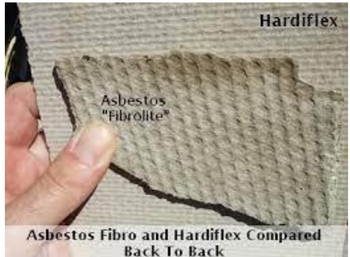
Notice the dimple pattern on the asbestos fibro when compared to modern non-asbestos Hardiflex
